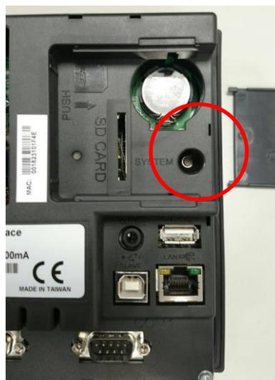
Note: The system button is hidden under the battery cover with the 7 and 8 inch models.
