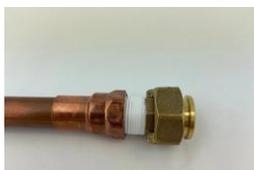
NOTE: Meter spuds are NPSM-straight threads. NPT taper threads cannot be connected directly with the meter spuds. You must use the couplings which come with the meter to connect them.
