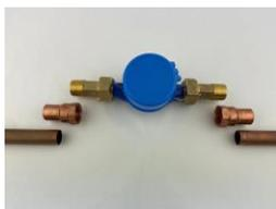
1. Mark the pipe at a location at least 10 diameters of straight pipe at the inlet and 5 diameters at the outlet to assure proper flow profile to the meter
