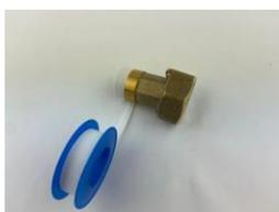
5. Wrap Teflon tape onto coupling tailpiece to a length of at least 5 threads. Place coupling tailpiece through center of nut. Hand tighten coupling tailpiece to pipe fitting.
