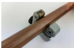
2. Where the pipe is marked, use a tubing cutter to remove the required pipe length.
