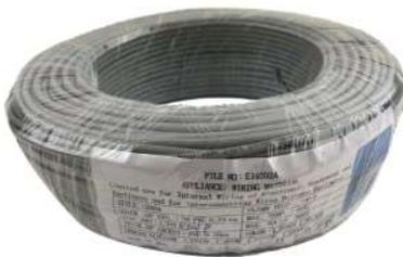
To securely transfer metering data for DAE Cloud Metering Solutions on Water, please use UL2464 cable to extend connection between water meters (have about 4 ft pulse cable) and AMR130AN or reading of Cell phone/PC may be more than the reading of meter due to exterior interference. With UL2464 cable, connection between meter, AMR130AN can be extended at least 328 ft, and at least 2000 ft between CC2030 and AMR130AN.
