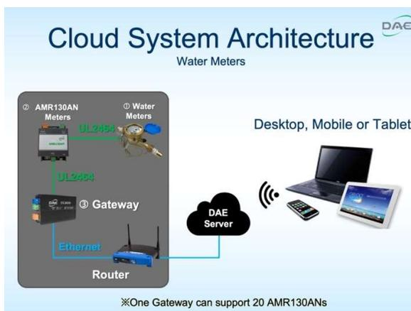
**1 DAE CC2030 KIT Gateway + 1 AMR130AN KIT** can read 1 water meter with pulse output (like DAE MJ-75n, PD-75, V-75P, VM-75P, and WP-200P) remotely with cell phone, PC and generate billing report. One CC2030 Gateway can monitor 20 meters (water, electricity, and gas).
