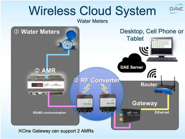
For existing building, hard to draw cable between AMR (close to water meter) and CC2030 (close to your router), please choose **1 AMR KIT + 1 CC2030 KIT + 2 WSC500 RF Converter** to connect them wirelessly.
