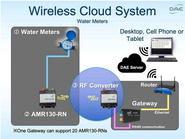
For existing building, hard to draw cable between AMR130AN (close to 1 water meter) and CC2030 (close to your router), please choose **1 AMR130-RN KIT + 1 CC2030 KIT + 1 WSC500 RF Converters** to connect them wirelessly.
